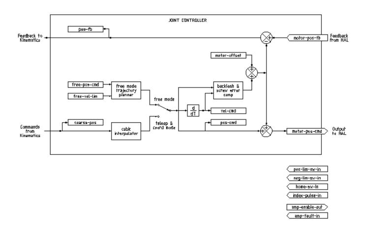
Figur 3.1: Joint Controller Block Diagram
