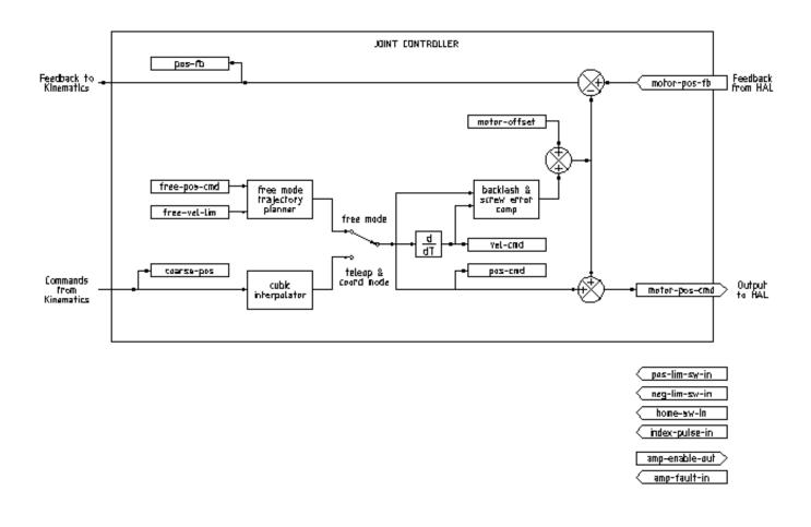
**Joint Controller Block Diagram** The above figure shows five of the seven sets of position information that form the main data flow through the motion controller. The seven forms of position data are as follows:
