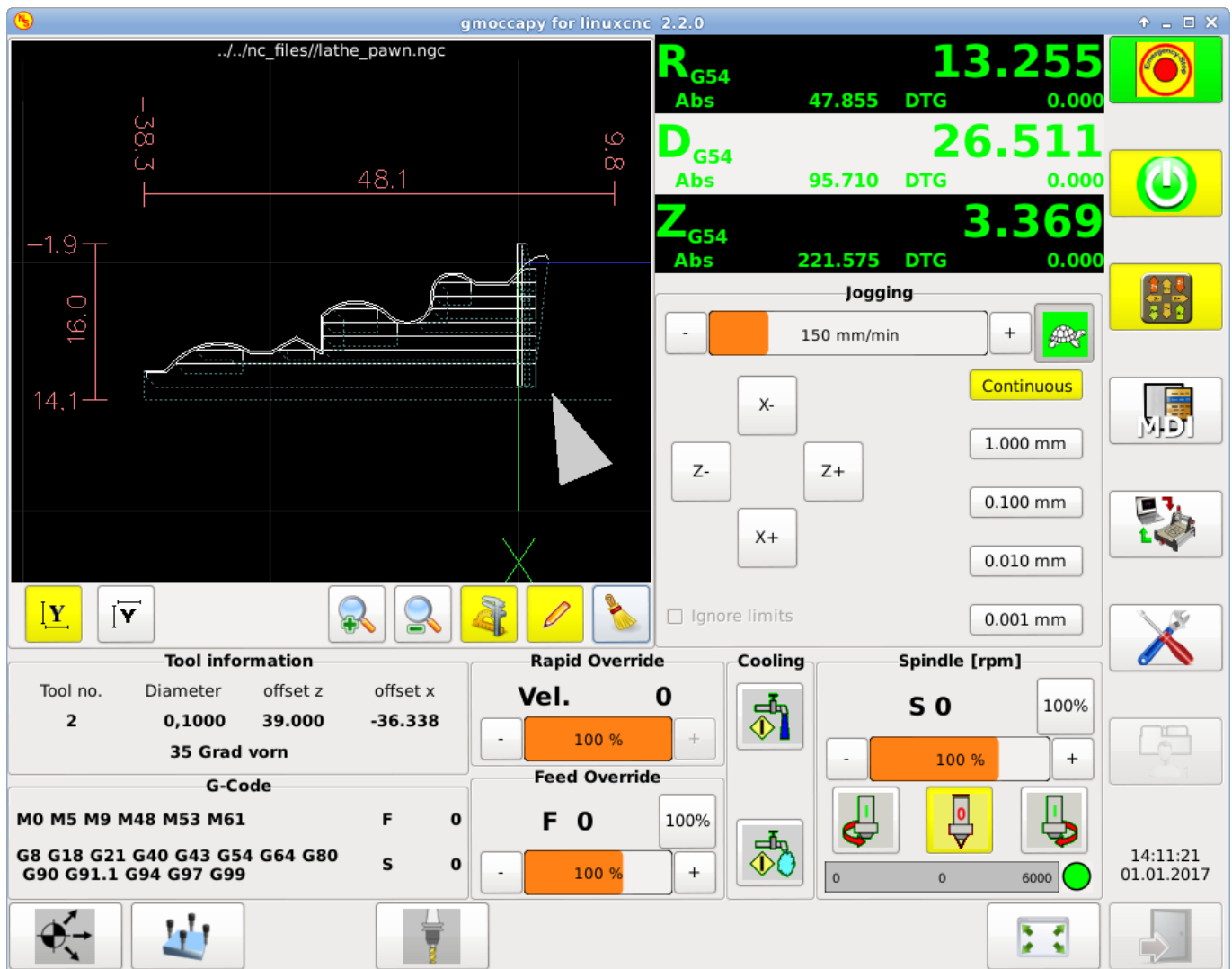
Figure 4.14: Normal Lathe
