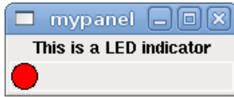
Figure 12.2: Simple PyVCP LED Panel Example
