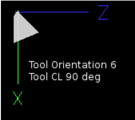
Figure 20.3: Tool Positions 5, 6, 7 & 8
