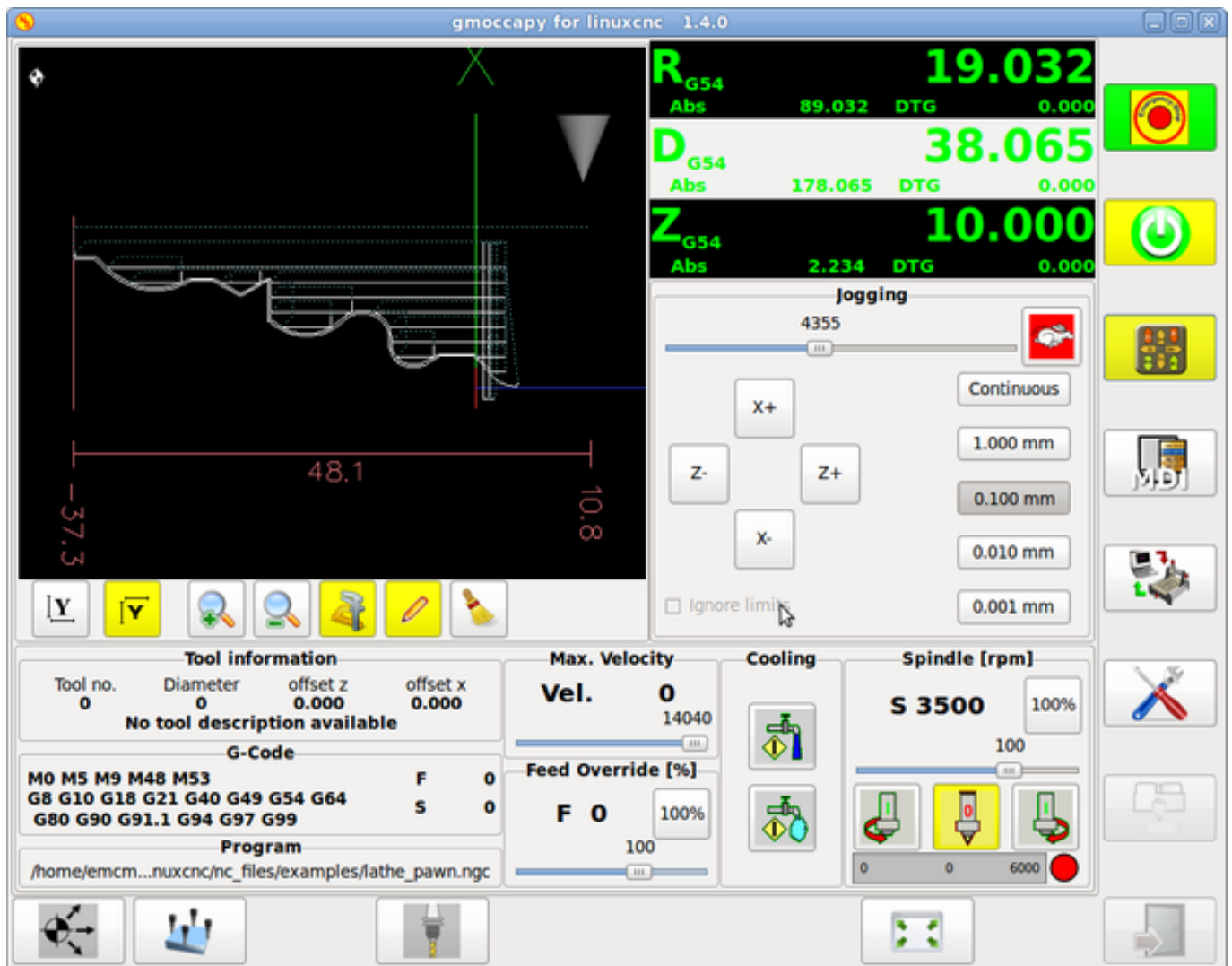
Figure 4.14: Back Tool Lathe
