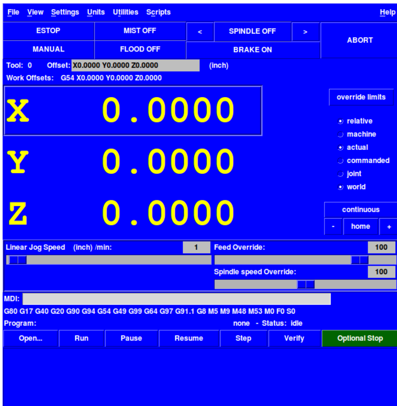
Figure 2.6: The TkLinuxCNC GUI
