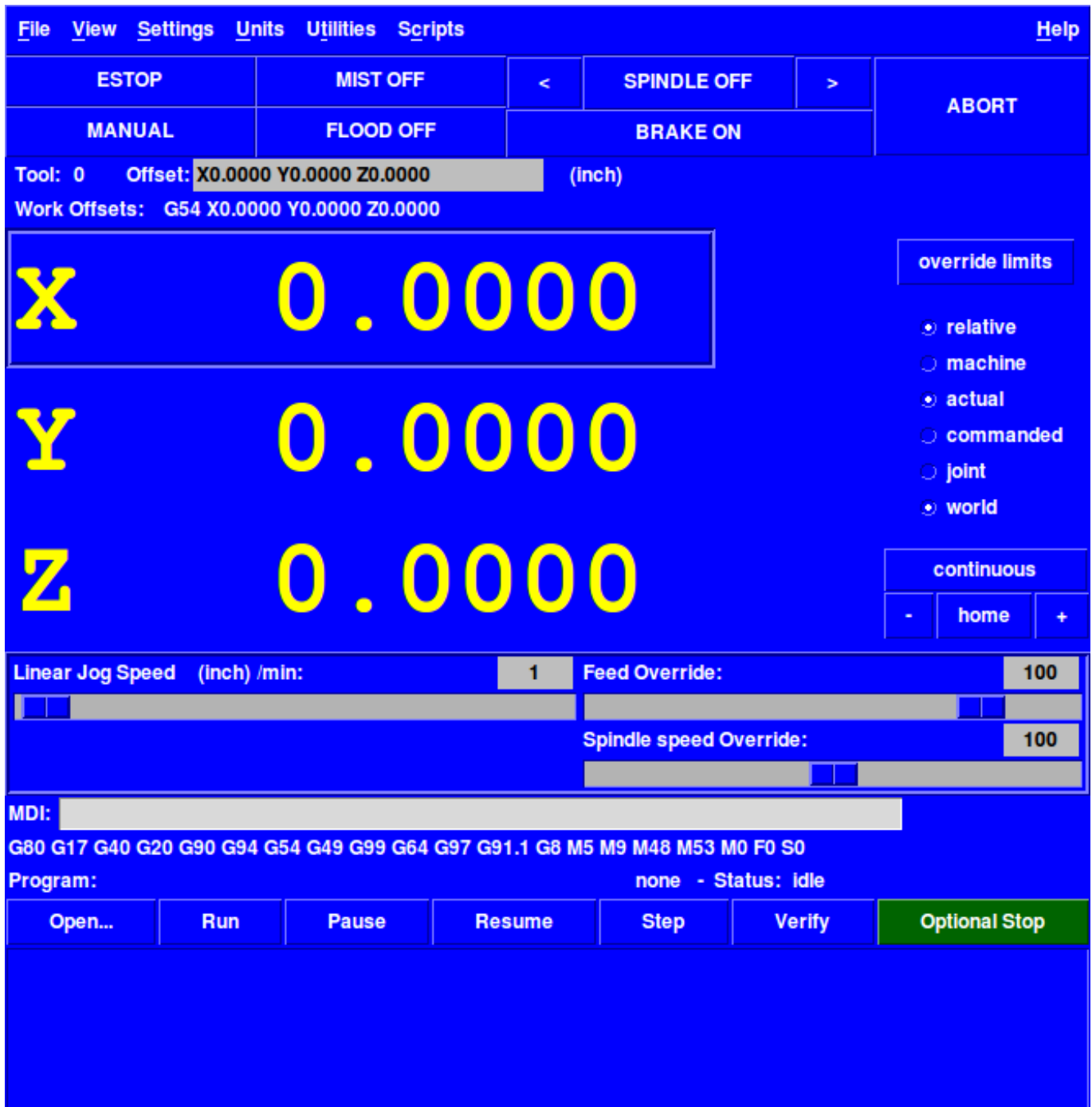
Figure 2.6: The TkLinuxCNC GUI
