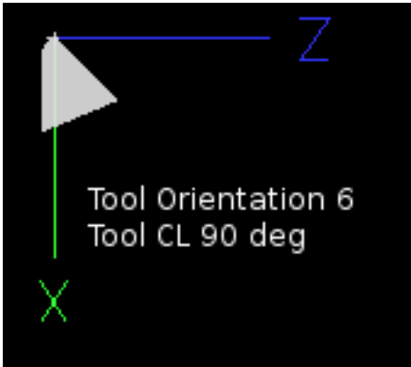
Figure 19.3: Tool Positions 5, 6, 7 & 8
