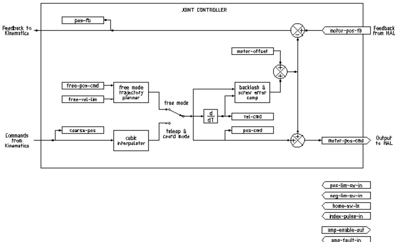
**Joint Controller Block Diagram** The above figure shows five of the seven sets of position information that form the main data flow through the motion controller. The seven forms of position data are as follows:
