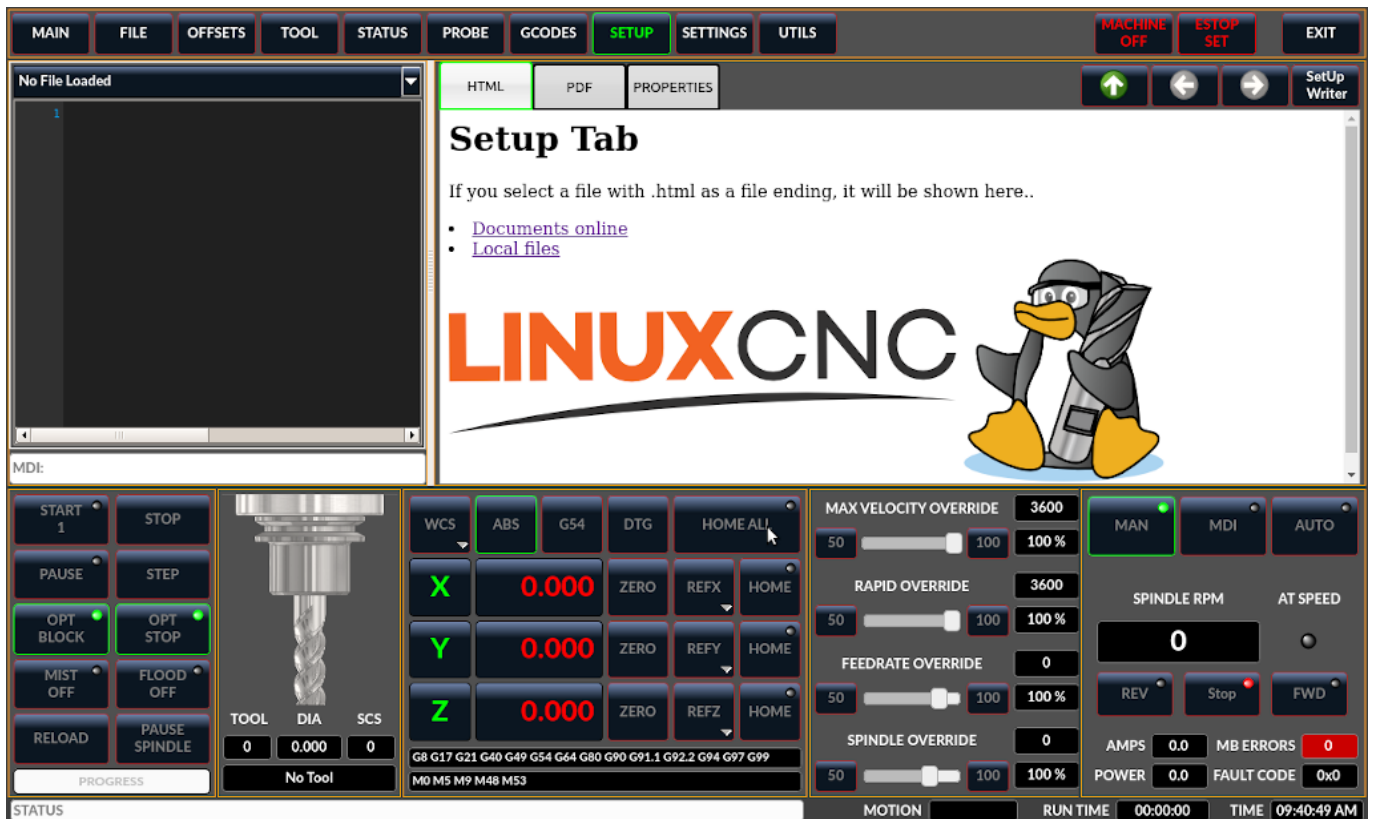
Figure 10.34: QtDragon - Setup Tab Sample
