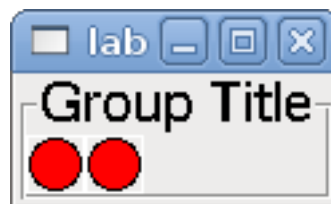
Figure 12.27 - Simple labelframe Example
