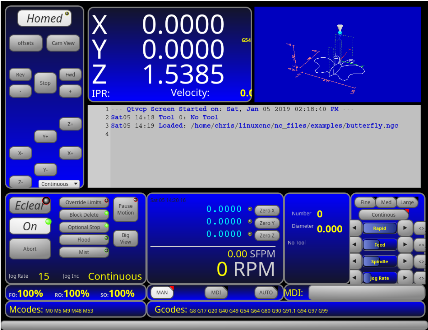
Figure 12.56 – QtDefault - 3-Axis Sample
