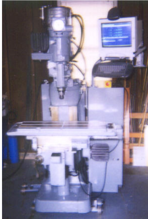
Figure 1. Open Engineering's Bridgeport three-axis knee mill retrofitted with the EMC. 5
