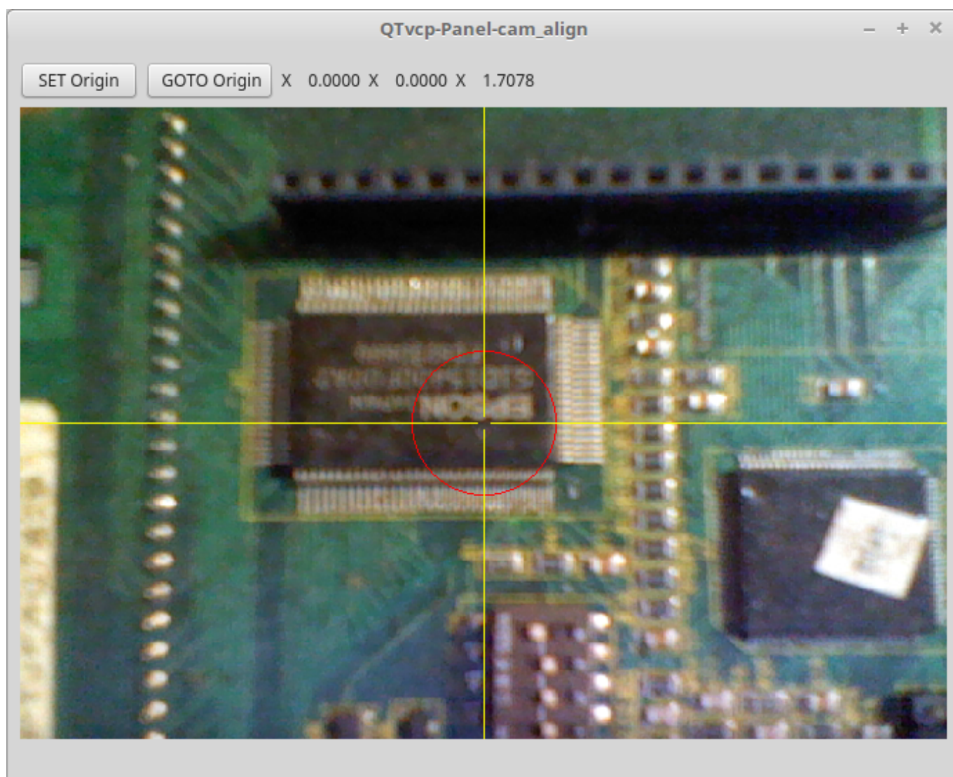
Figure 12.63: cam_align - Camera Alignment VCP
