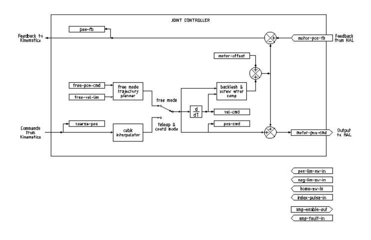
Figure 3.1 - Joint Controller Block Diagram
