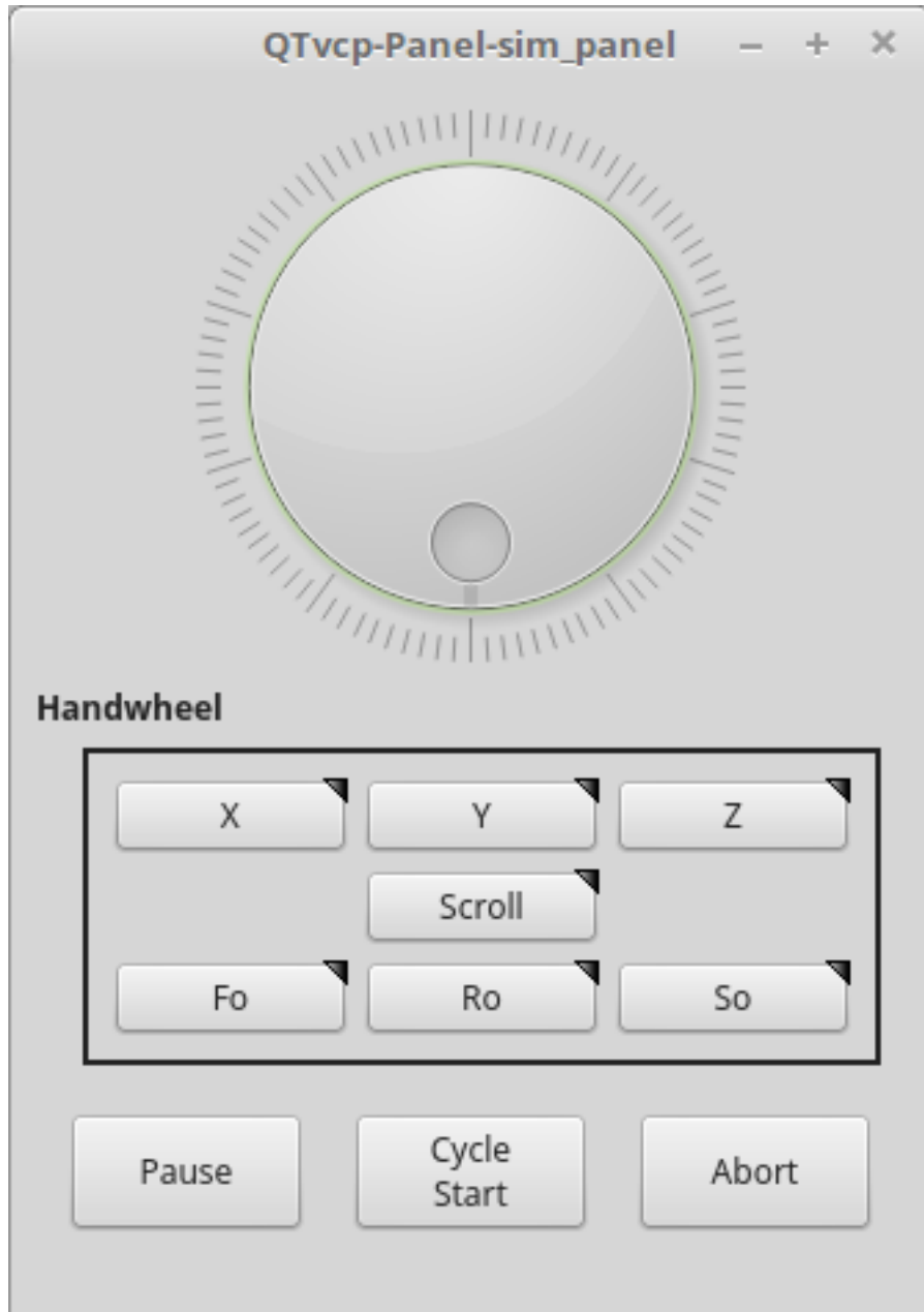
Figure 12.64: QtVCP Sim Builtin Panel
