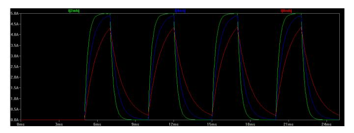
The accepted way of improving motor speed while maintaining torque is to increase the speed at which the magnetic field of the motor coils can expand and collapse. The easiest way to accomplish this is to increase the supply voltage to force the current in each winding to rise and fall much more rapidly. A quicker magnetising time equates to faster step rates while improving torque at higher speeds, both of which are obviously desirable in a CNC system.
