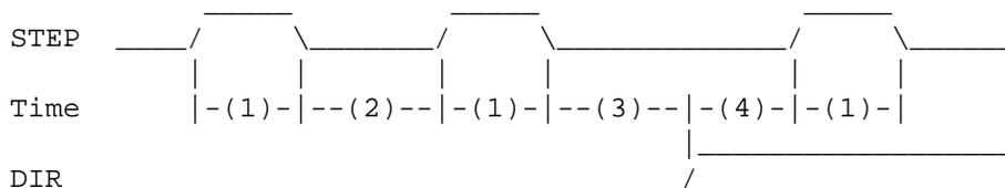
For step type 1, timing parameters 1, 2, and 5 are used. The following timing diagram shows the output waveforms, and what each parameter adjusts.
