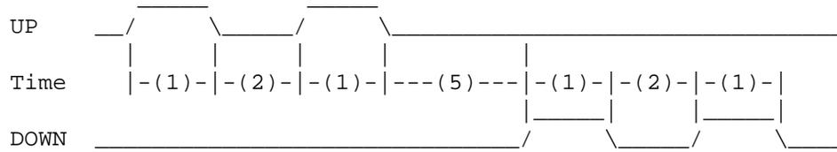
For step types 2 and higher, the exact pattern of the outputs depends on the step type (see the HAL manual for a full listing). The outputs change from one state to another at a minimum interval of **steplen**. When a direction change occurs, the minimum time between the last step in one direction and the first in the other direction is the sum of **steplen** and **dirdelay**.
