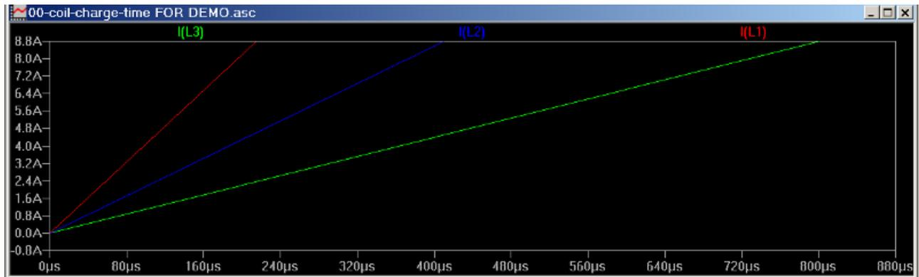
By 80  $\mu$ s (microseconds) the 2 mH coil has achieved 3.2 Amps. At that same time, the 8 mH coil has only achieved about 0.9 Amps. If the stepper motor is rated at a certain torque at 3 Amps, but it only gets to 0.9 Amps it would seem like you have a little less than 1/3 of the rated torque at 80  $\mu$ s per step, but it's even less than that, since it only starts exerting that 1/3 torque at the 80  $\mu$ s mark. At 40  $\mu$ s it may only be delivering 1/6 of the full rated torque.
