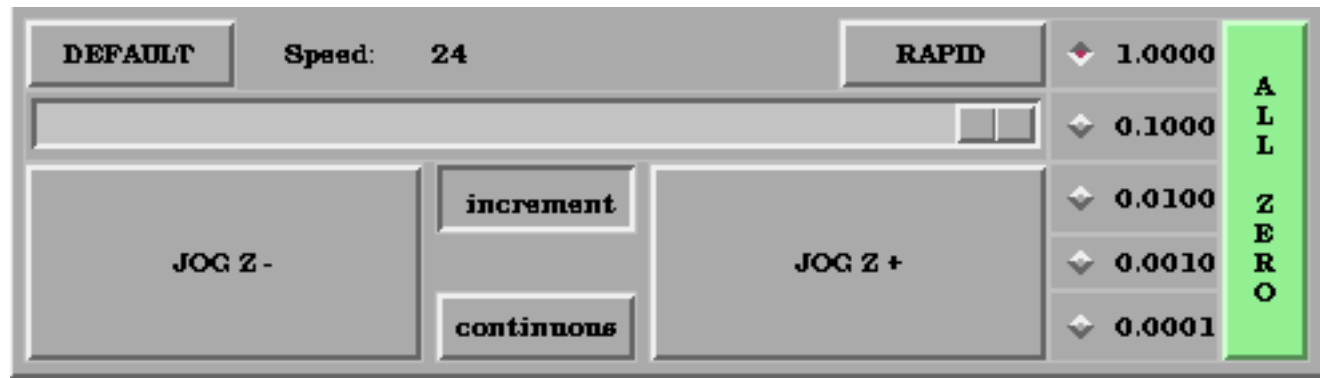
Figure 2.24: Manual Mode Buttons
