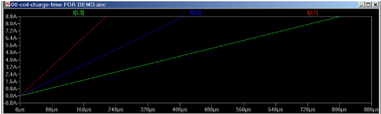
By 80 uS (microseconds) the 2 mH coil has achieved 3.2 Amps. At that same time, the 8 mH coil has only achieved about 0.9 Amps. If the stepper motor is rated at a certain torque at 3 Amps, but it only gets to 0.9 Amps it would seem like you have a little less than 1/3 of the rated torque at 80 uS per step, but it's even less than that, since it only starts exerting that 1/3 torque at the 80 uS mark. At 40 uS it may only be delivering 1/6 of the full rated torque.
